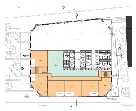
Image 14: Sketch arrangement of first floor residential plan
